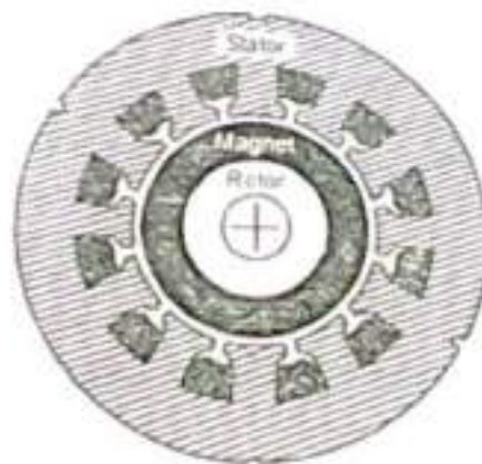
Fig 4.1 Arrangement of permanent magnet in the rotor
